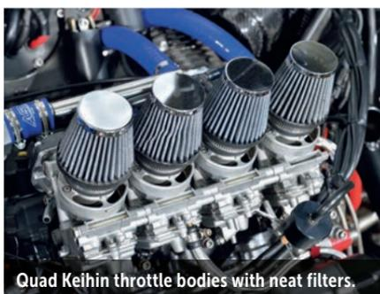
Quad Keihin throttle bodies with neat filters.
